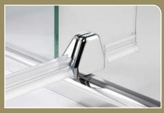
The 'lowering' and 'offset' effect of the design automatically reduces the gap between door and sill on door closure. When in the closed position the shower door is located inside the shower recess, ensuring water runoff is directed back into the shower enclosure, helping minimise splashing further enhancing water resistance.
